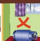
Never roll the cylinder in a horizontal position.
