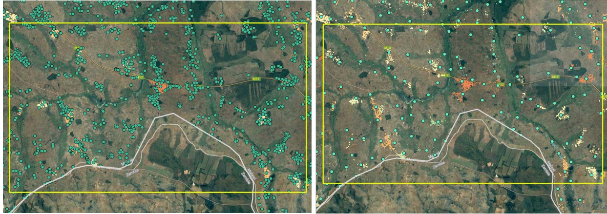
Figure 8: Identification of centroids within gridded polygons (left) followed by clustering of centroids to form potential transformer sites with 500 m coverage area (right).
